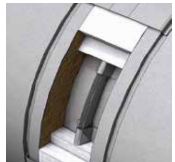
Flange connection secured by internal V-band and locking band 2.0 in the external
